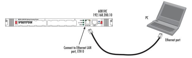
Figure 11. Connecting the 6081RC to your laptop PC via the Ethernet port
